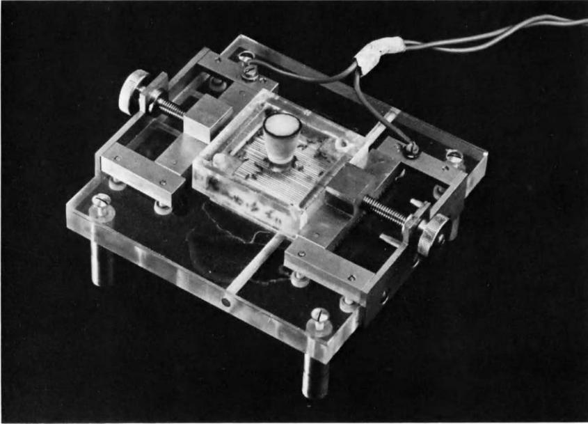
**Fig. 4** Apparatus for the collection of venom from the wasp *Microbracon hebetor* by electrical stimulation. From Piek (1966).
