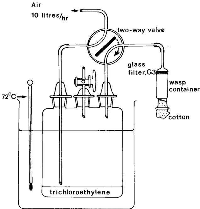
**Fig. 6** Equipment for the collection of venom from the wasp *Microbracon hebetor*, using trilene, according to the method described by Drenth (1974).
